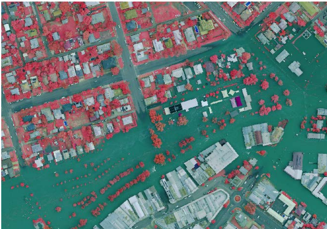
Image 3: 150mm RGBN imagery displayed as false-colour infrared with an NRG band combination
