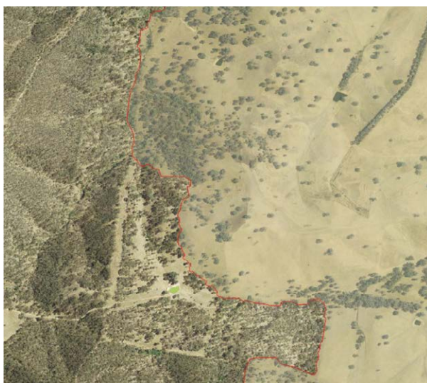
Image 4: Mismatch in terrain reflectance due to differing atmospheric conditions between flight lines
