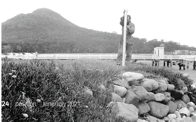
Left and right: Levelling at the Port Stephens, NSW, tide gauge. Courtesy of DCS Spatial Services.
