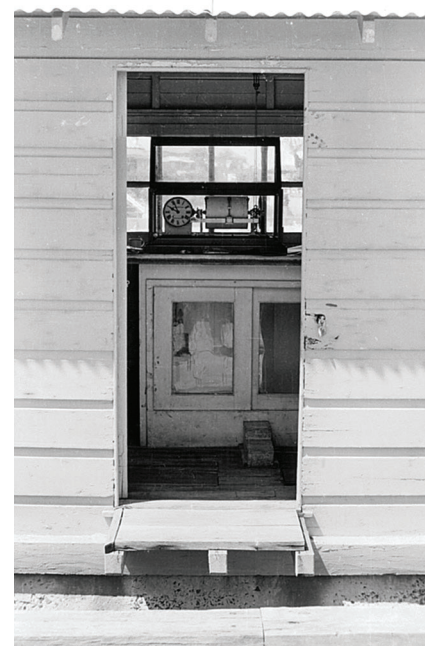
Above and below: Camp Cove tide gauge in Sydney, showing the recorder hut housing a Harrison tide recorder.
