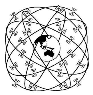
Each satellite whizzes around about 20 200 kilometres above the Earth's surface. That's about the same distance as from the South Pole to the North Pole, the long way ... but straight up! This incredible altitude, and the birdcage pattern of orbits allows us to 'see' between four and ten satellites at any time, from anywhere on the globe.
