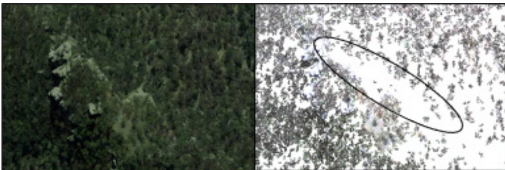
Data voids on steep slopes
