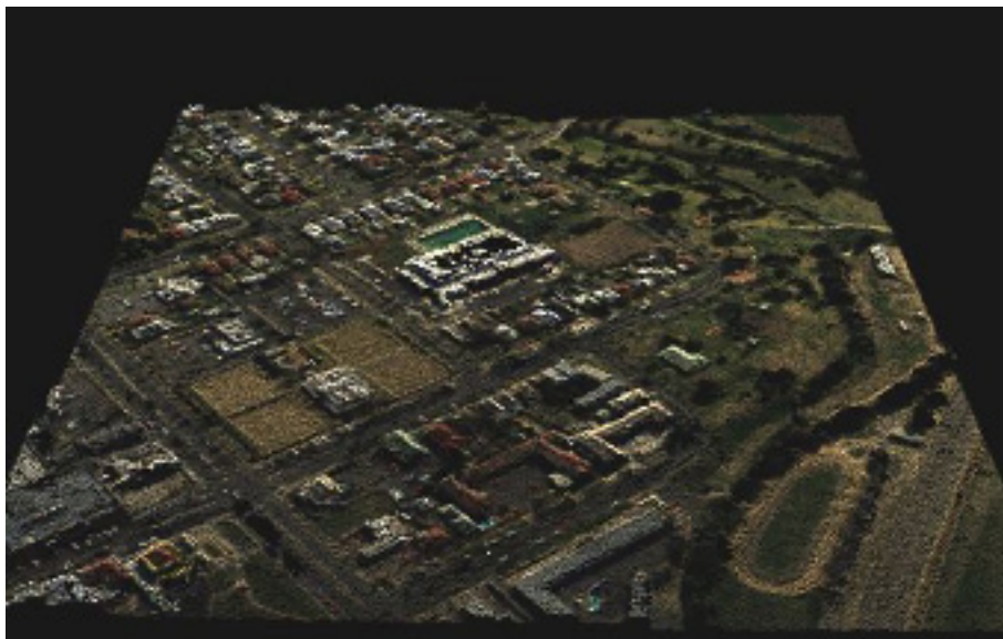
3D visualisation of unclassified point cloud displayed by RGB values
