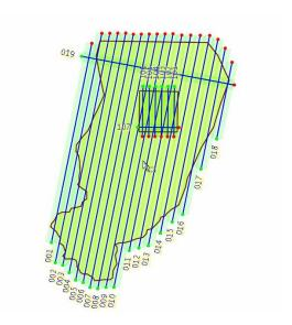
Figure 3: Glen Innes survey of 9 June 2009 showing the distribution of reference stations with baseline lengths and the survey area with (numbered) flight runs.
