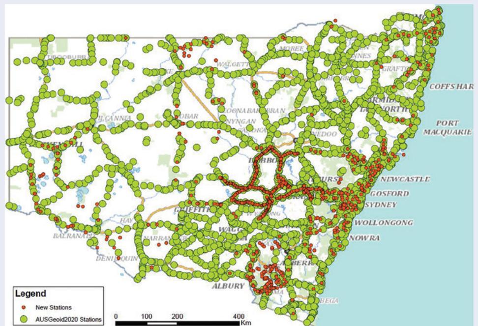
Figure 1: GNSS datasets of at least 6 hours duration on levelled marks observed by DCS Spatial Services, including those contributing to AUSGeoid2020.
