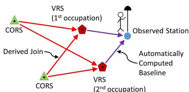
Figure 4: NRTK automatic baseline network being connected to datum via a join between each VRS and the two nearest CORS.
