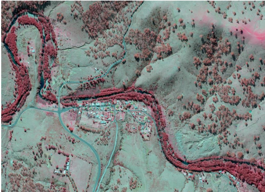
50cm BGRN imagery displayed as false-colour infrared with an NRG band combination.
