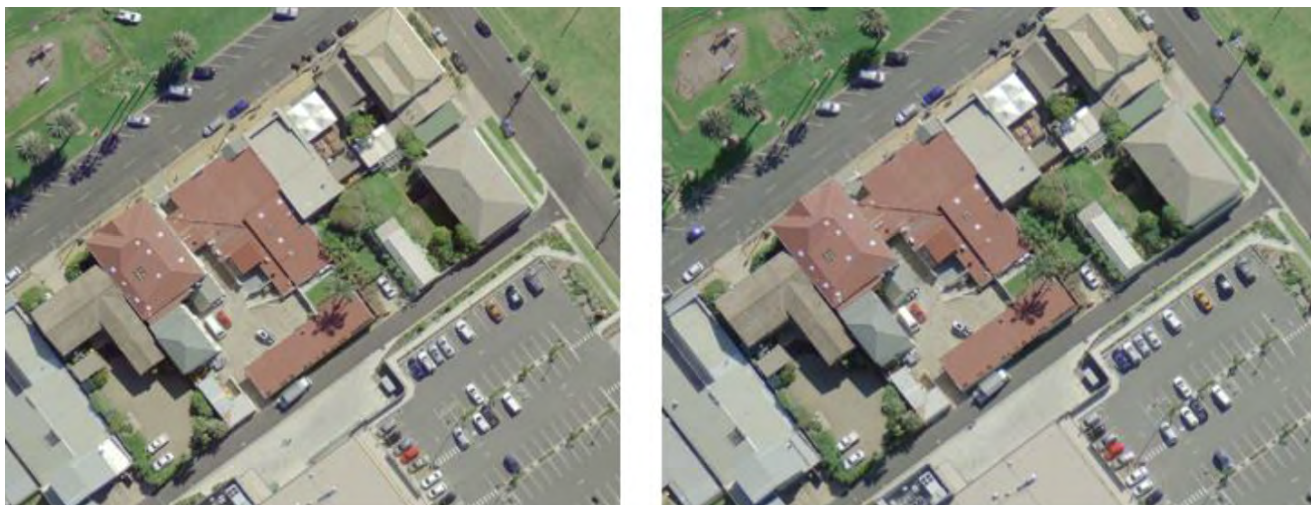
Images depicts a sample of the Standard Aerial Imagery Stereo Workspaces dataset (Left: Nadir look-angle imagery, Right: Backwards look-angle imagery) © DCS Spatial Services 2023
