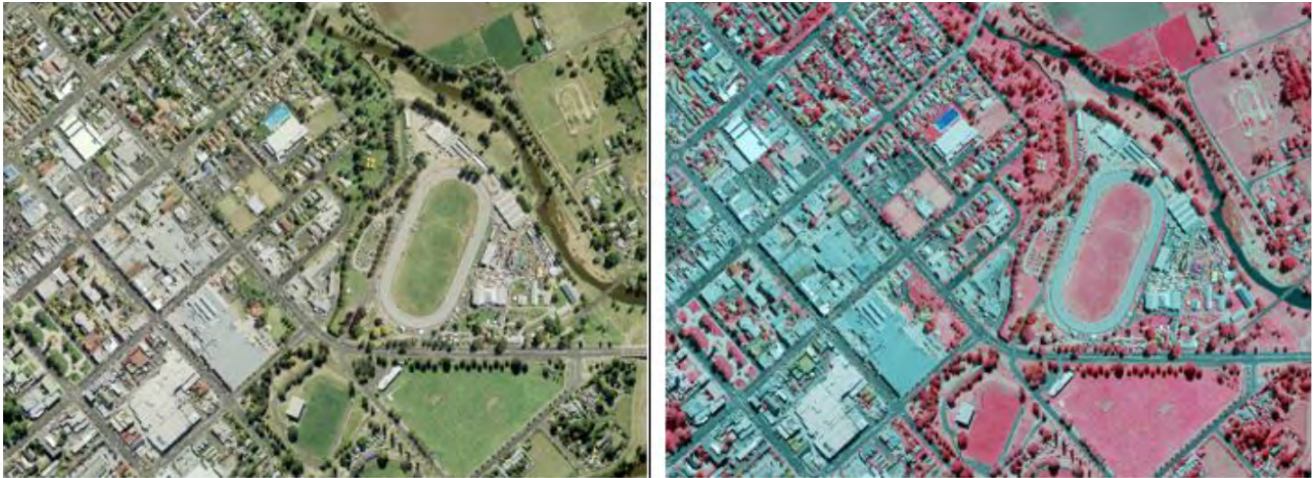
Images depict samples of airborne imagery over Bathurst, NSW (left) at 10cm in RGB and CIR (Left) © Spatial Services 2023
