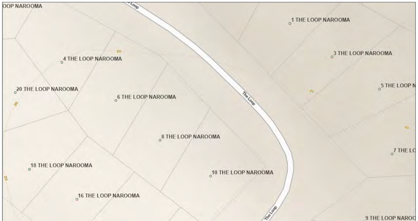
Image depicts Address Points labelled with House numbers and situated at centroid of Property. NB Building Address Points are displayed in brown colour and are situated over buildings © DCS Spatial Services 2023
