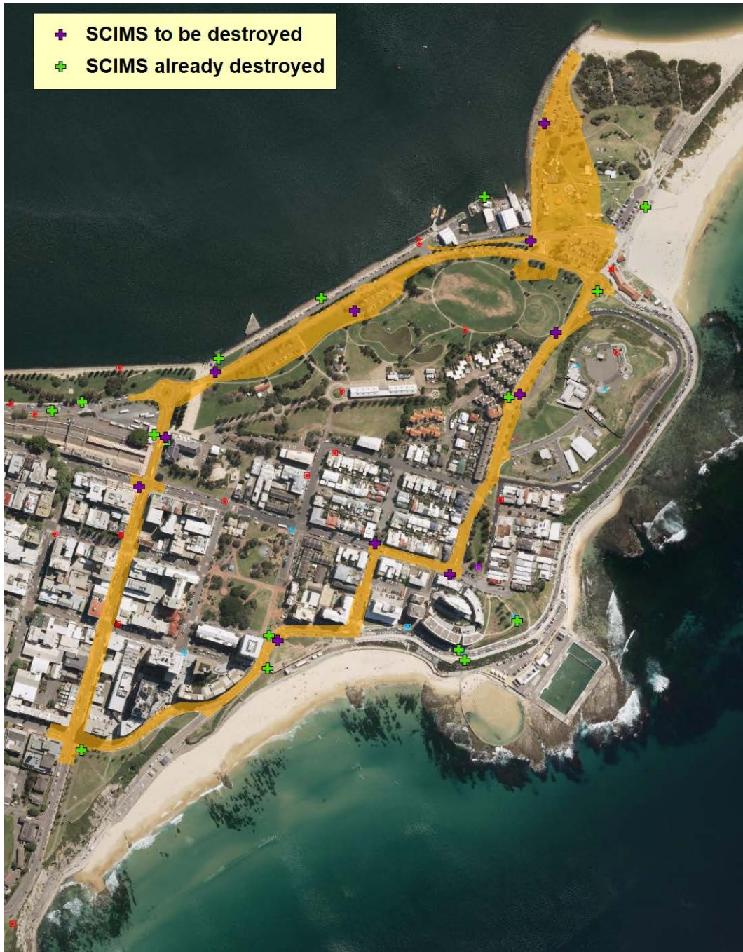
Figure 4: SCIMS marks already destroyed and to be destroyed.
