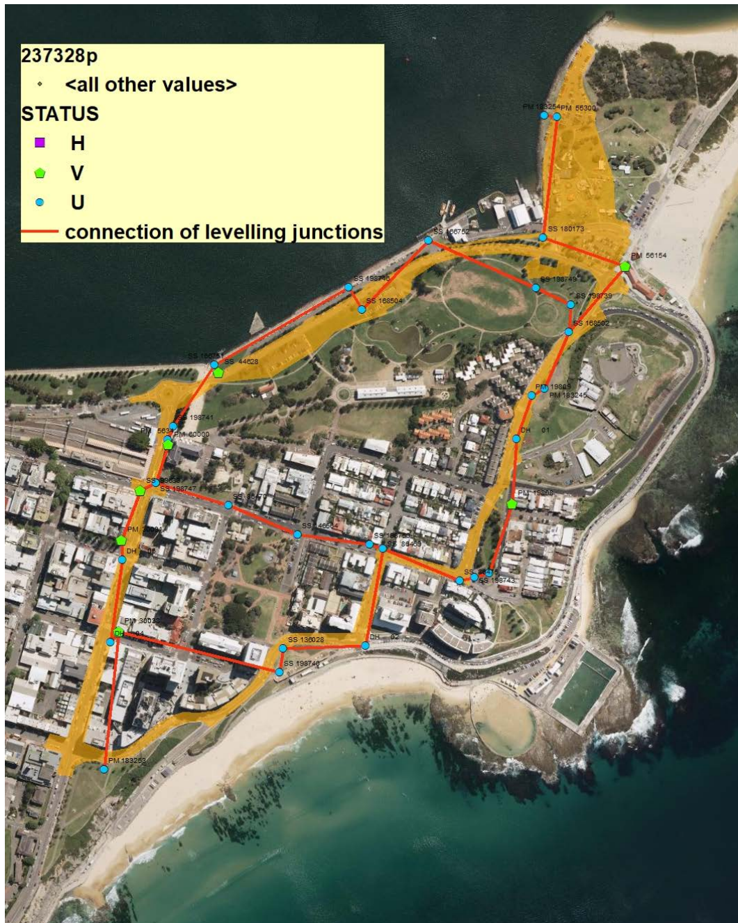
Figure 6: Vertical levelling network.
