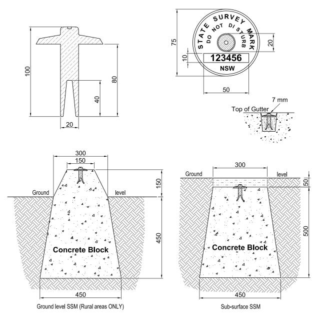
NOTE: Where an existing structure or solid rock is unavailable the mark is to be placed in the top of a concrete block and cast in situ. The block must have a volume of concrete of at least 0.07 cubic metres and shaped as indicated above
