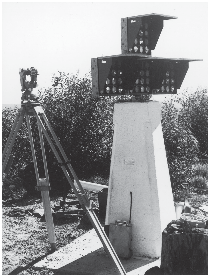
Concrete Pillar - these trigonometrical stations were introduced in the 1970's to replace the rock cairn. Here a set of 64 prisms and a Wild T2 theodolite are being used for simultaneous reciprocal vertical observations prior to EDM measurement.
