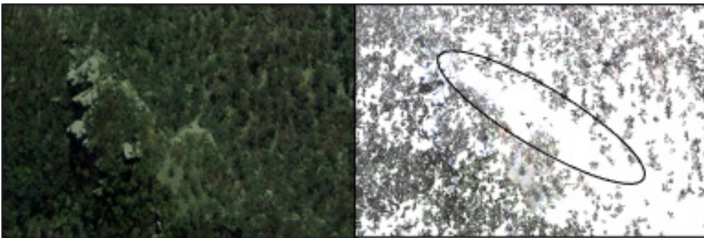
Data voids on steep slopes
