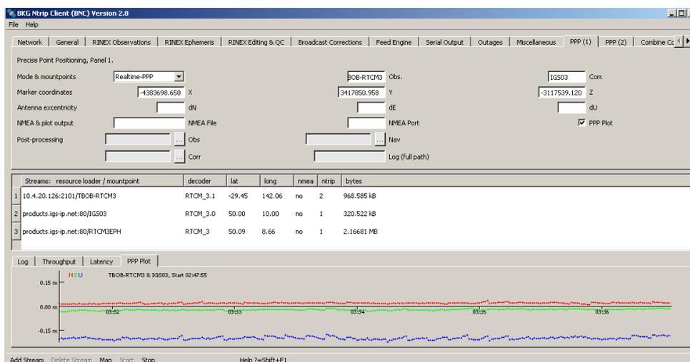
**Figure 3:** Example of a PPP engine solution on the BKG Ntrip Client (BNC) Version 2.8
