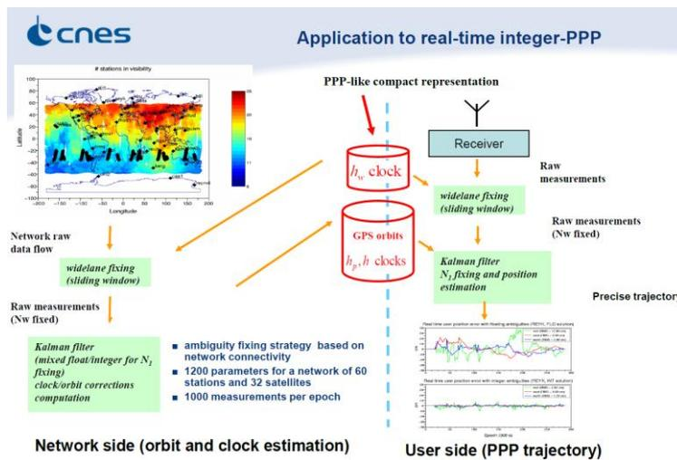
**Figure 4:** Diagram of the architecture of the CNES demonstrator (Laurichesse, 2011).
