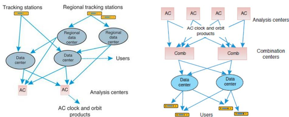
**Figure 2:** IGS GNSS data centre and product distribution architecture (Caissy *et al.*, 2012).
