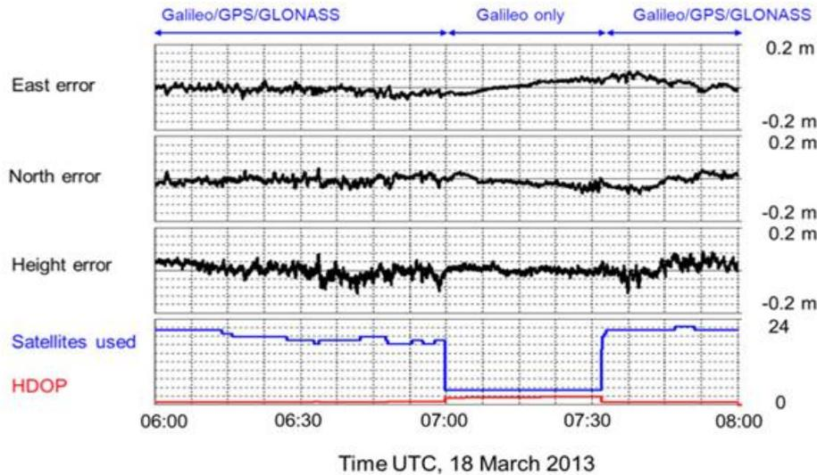
**Figure 9:** Accuracy of the Galileo/GPS/GLONASS solution at a station in Oslo, Norway over a 2-hour time period (GPS World Staff, 2013).
