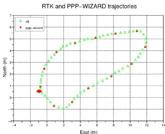
**Figure 8:** Antenna trajectories of RTK and PPP-wizard (Laurichesse, 2011).
