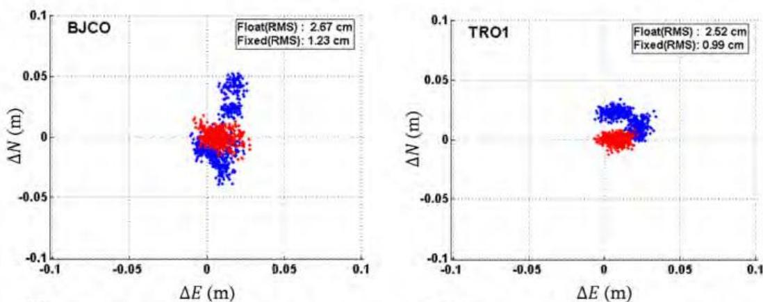
Figure 6: AR PPP (Red) Vs Float PPP (Blue) accuracy for station BJCO and TRO1 using Nexteqs FCB estimates from a global network of stations (Urquhart *et al.*, 2012).
