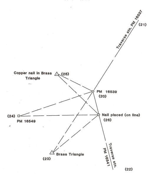
From occupied station PM 16539 (20) measure directions (21), (22), (23), (24), (25) and (26) on F.L. and reverse on F.R. Measure distances (23), (24), (25), & (26). Record directions (22) and (26) separately.
