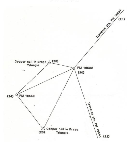
From occupied Station PM 16539 (20) measure directions (21), (22), (23), (24) and (25) on F.L. and reverse on F.R. Measure distances to (23), (24) & (26).
