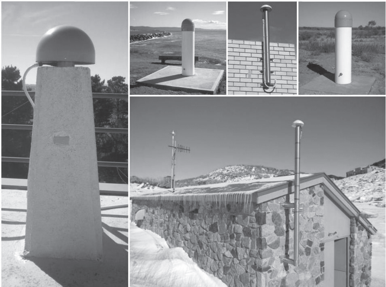
Various Continuously Operating Reference Stations in the CORSnet-NSW network.
