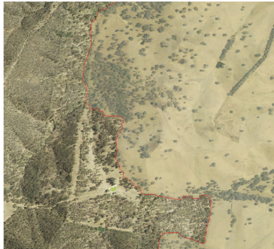
Mismatch in terrain reflectance due to differing atmospheric conditions between flight lines.
