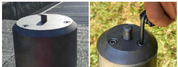
Figure 6: Adjustment of the CAAM, integrated into the GNSS antenna monument.
