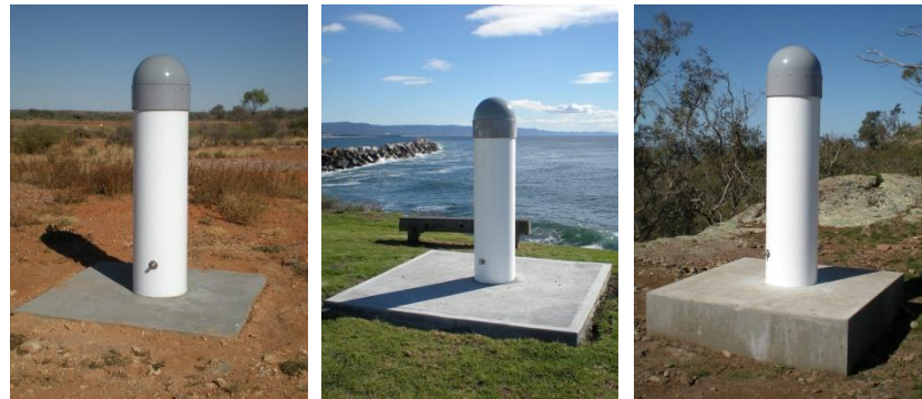
Figure 3: Typical CORSnet-NSW Tier 2 antenna monuments.
