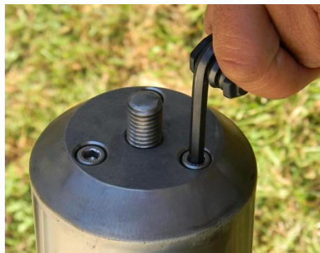
Figure 11: CORSnet-NSW Adjustable Antenna Mount (CAAM), integrated into the GNSS antenna monument.
